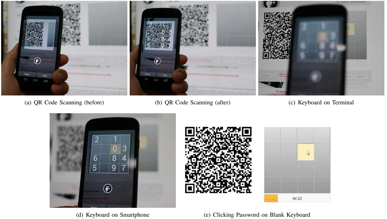
Fig. 2. Photographs of the prototype we have developed to demonstrate our authentication protocols. (a) and (b) show the moments of a QR code scanning of a keyboard layout. (c) shows the blank keyboard shown at the terminal (on LCD screen). (d) shows the decoded randomized layout of the keyboard obtained from the QR code after decryption as viewed on smartphone. Note that the yellow square on which the mouse cursor is hovering in the terminal is shown through the smartphone to assist user's input. (e) shows that a user is clicking the password on the blank keyboard while seeing numbers through the smartphone.
